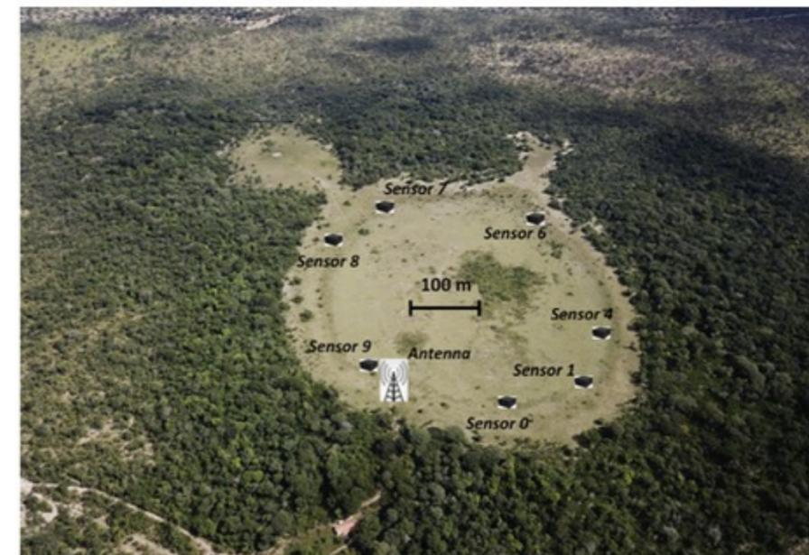
Fig. 1 – Photo of the location of H<sub>2</sub> monitoring in a circular depression of the São Francisco Basin (Brazil). H<sub>2</sub> sensors positions, and the data-transmitting antenna are shown.
